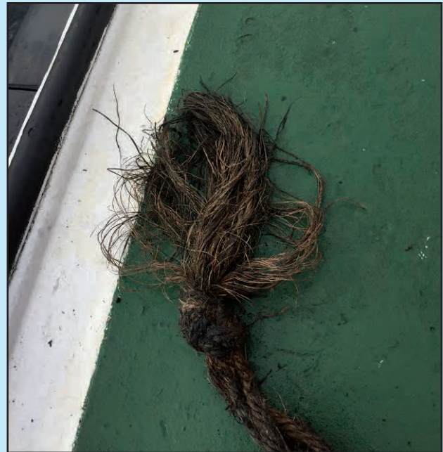
Figure 3: Ladder side rope showing contamination
