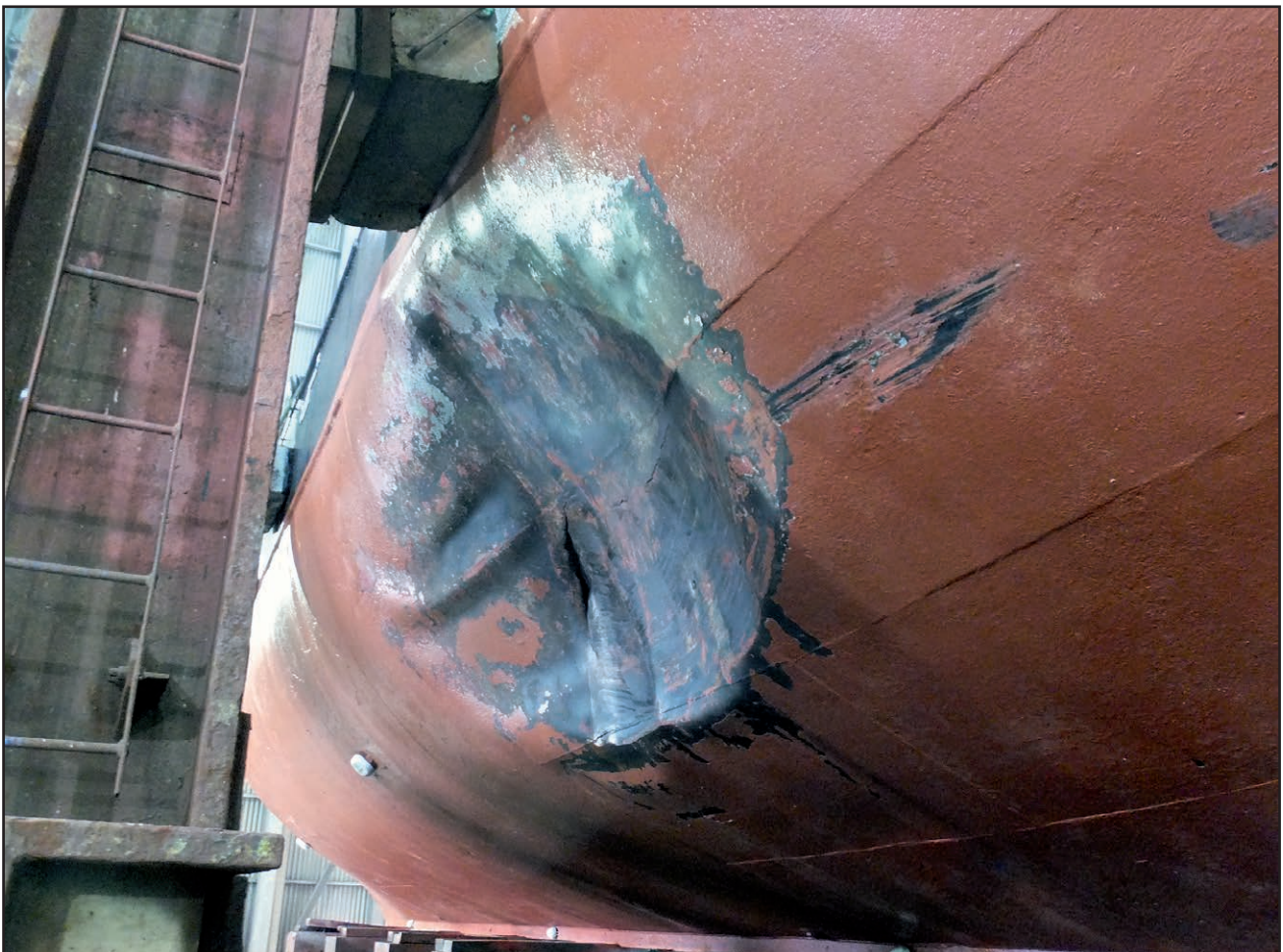
Figure: Indentation in the bunker barge's hull caused by the cargo ship's bulbous bow
