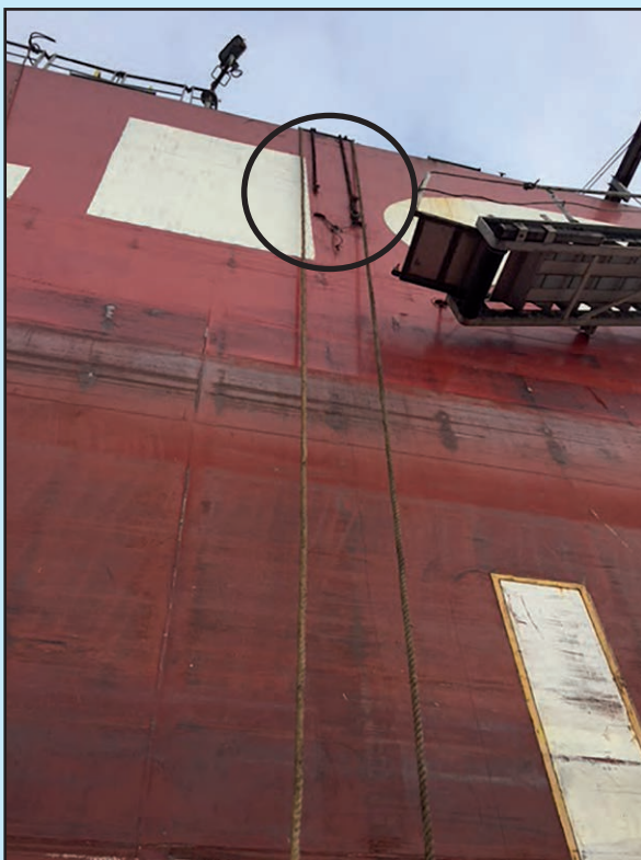
Figure 2: Ladder rigged position, showing broken section
