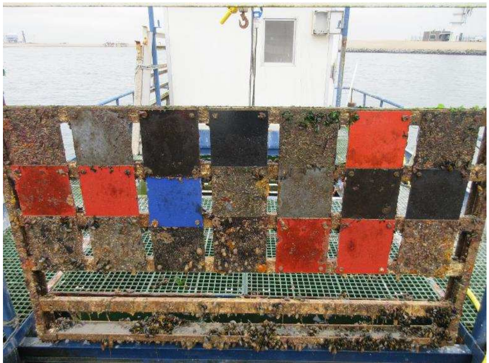
Figure 16. Panels with antifouling products at fourth inspection on September 24, 2019.
