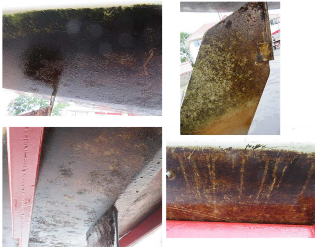
Figure 28. Compilation of pictures of the hull condition of a boat without antifouling at the fresh water location in Heeg.
