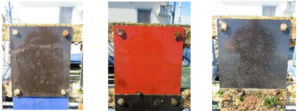
Figure 11. Detailed pictures of panels with Renolit, Silic One and Bioclean (from left to right).
