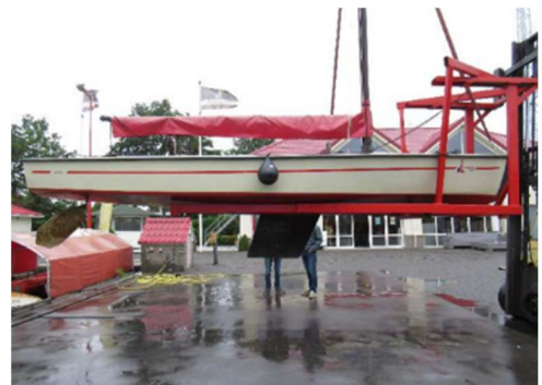
Figure 4. Illustration of boat lifting process at fresh water location Ottenhome in Heeg.
