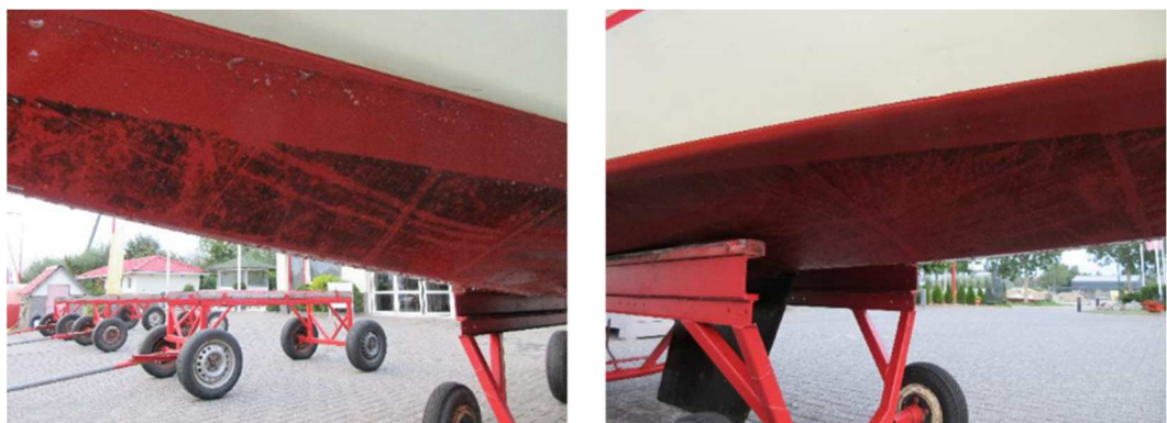
Figure 25. Boat with MacGlide™ Pyramidal foil at the final inspection.
