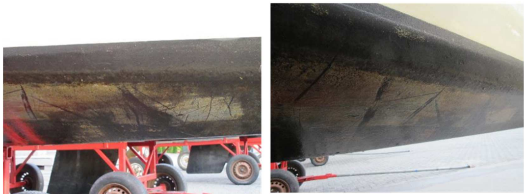
Figure 22. Boat with Melkfett product at the final inspection.
