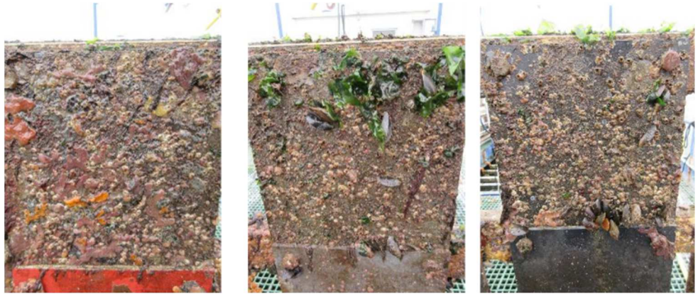
Figure 17. Detailed pictures of panels with PVC, GPN and Seajet ex3 (from left to right).
