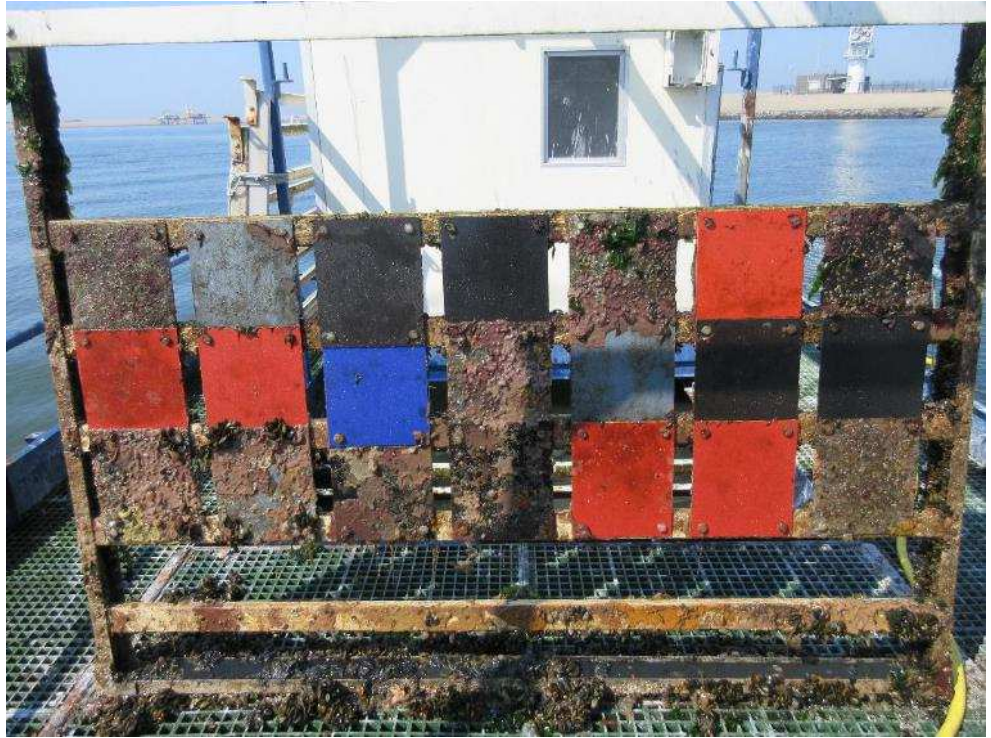
Figure 13. Panels with antifouling products at third inspection on August 26, 2019.
